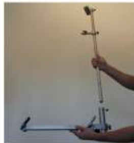
Undo the Bottom Clamp thumb screw and slide out the Main Rod.
