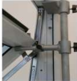
Close up view of the Friction Stay hitting the top of the inner frame.
