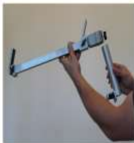
Remove the Bottom Clamp from the Bracing Arm.
